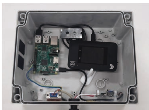
Figure 6) Components of a Next G telemetry system including the Next G modem, Raspberry Pi computer and cables that connect to the WoW indicator and power source.
